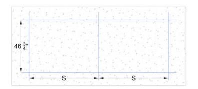
**ARRAY LAYOUT: MARK LOCATION OF ARRAY SUPPORTS.** EAST/WEST SUPPORT SPACING SHALL BE PER DESIGN AND ENGINEERING GUIDE. NORTH/SOUTH SPACING SHALL BE 46 3/4" TYPICAL.
